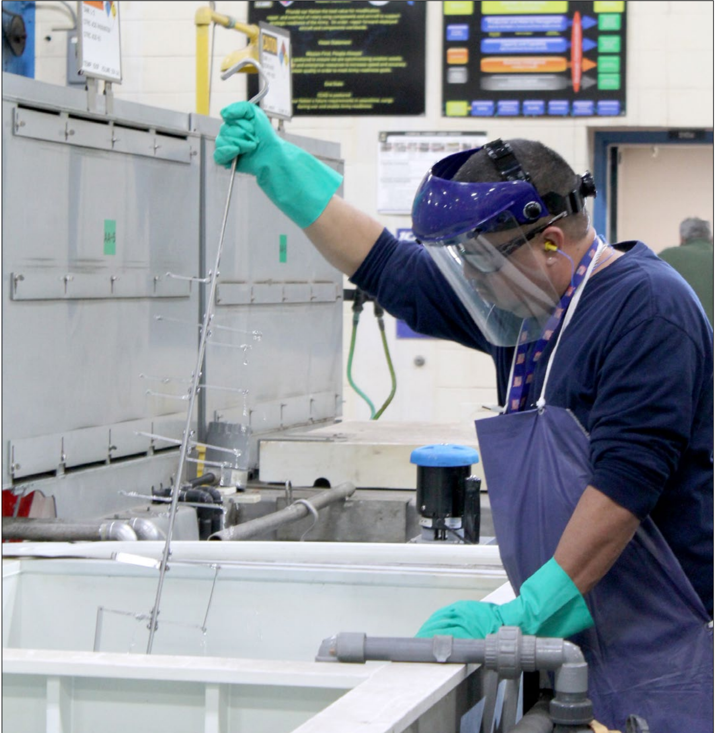
Adrian Alvarado passivates stainless steel alloy plates using a citric acid bath at Corpus Christi Army Depot in Texas as part of an NDCEE project to validate a more environmentally friendly process for increasing corrosion resistance for metals used in Army weapons systems. The citric acid passivation project was funded by the NDCEE in 2018 and completed in 2019.
