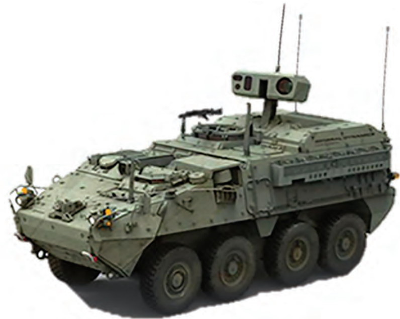
The MMHEL will demonstrate a Stryker-based HEL experimental prototype that is suitable for maneuvering Brigade Combat Teams and capable of countering UAS, RAM and ISR threats.
