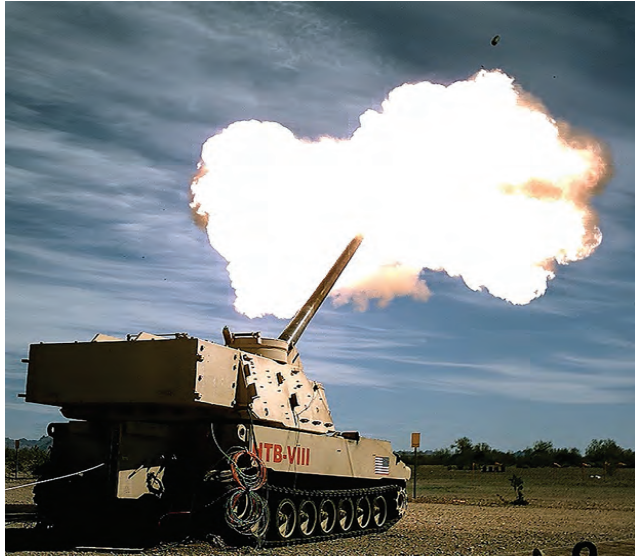
A prototype ERCA Howitzer test bed fires an XM1113 Rocket Assist Projectile. The Army is increasing its lethality overmatch for current and next generation 155 mm systems by developing lightweight armaments with improved accuracy, range and rate of fire.
