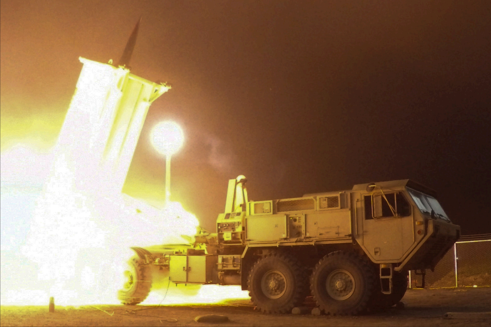
A Terminal High Altitude Area Defense (THAAD) interceptor is launched from the Pacific Spaceport Complex Alaska in Kodiak, Alaska, during Flight Experiment THAAD (FET)-01 on July 30, 2017 (EDT). During the test, the THAAD weapon system successfully intercepted an air-launched, medium-range ballistic missile (MRBM) target
