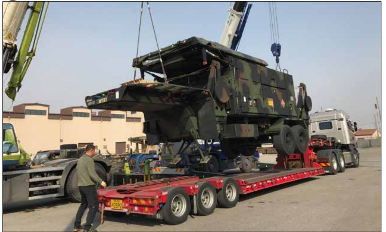
A radar system is lifted by two cranes and placed on a semitrailer at Osan Air Base, Jan. 26. The system will be transported to nearby Suwon Air Base to support 35th ADA Brigade as it conducts the largest Patriot modernization effort ever executed outside a depot facility. (Photo courtesy of Bryan Watkins)
