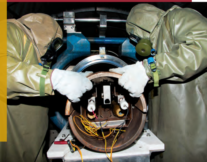
Two ECBC field operators prepare a recovered chemical munition for destruction in the Explosive Destruction System at Dover Air Force Base.
