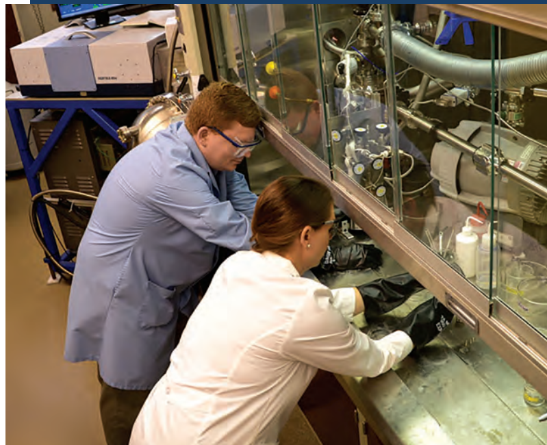
ECBC scientists built the built the surface science instrument which can safely perform ultra high vacuum studies with CWAs.
