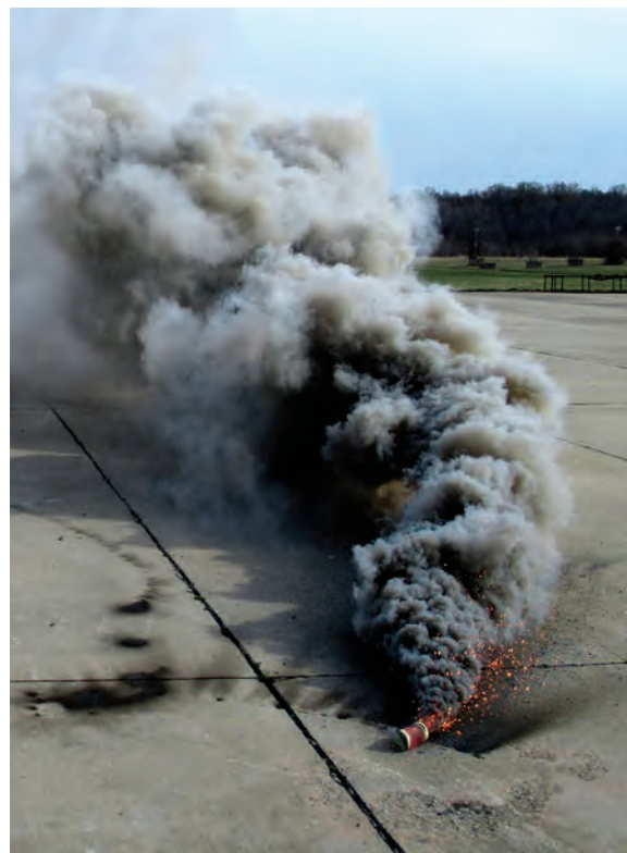
HX smoke creates a cloud that disperses better, stays suspended longer, and more effectively conceals Warfighters from the visual and infrared spectra.
