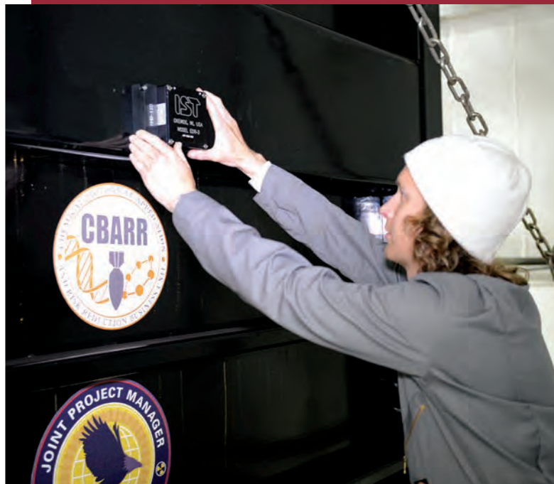
A MV Cape Ray crew member places a vibration sensor on FDHS equipment. ECBC engineers used vibration analysis to adapt the land-based FDHS for shipboard operations.
