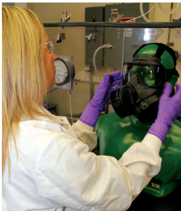
The silicon and butyl face piece of the M50 mask is flexible enough to fit all face sizes from the second to the 98th percentile of the adult population.
