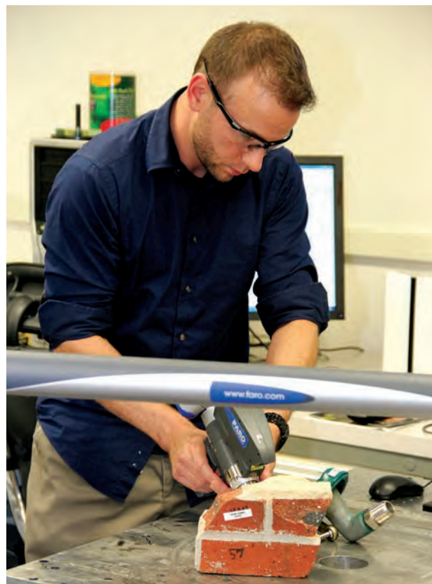
An ECBC technician scans a piece of a building in order to perform a 3-D blast reconstruction.
