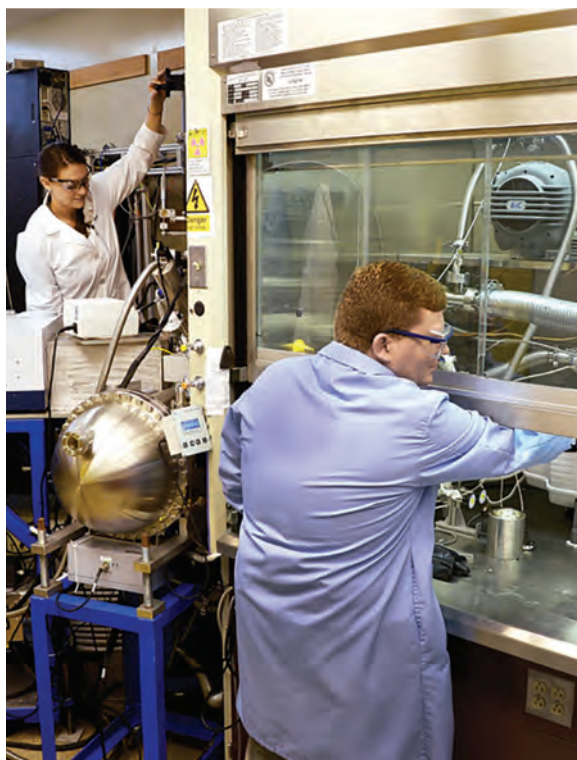
Working with scientists at Virginia Tech and private industry, ECBC has developed the nation's first chemical agent-permitted UHV system to advance the understanding of chemical warfare agent interactions with a material's surface at the molecular level.
