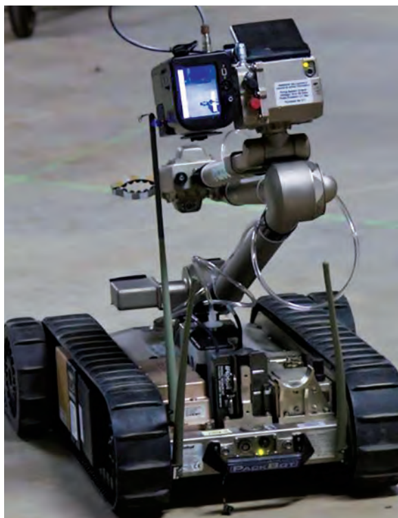
The RASR integrated into a robot allows for agent detection at extended ranges.
