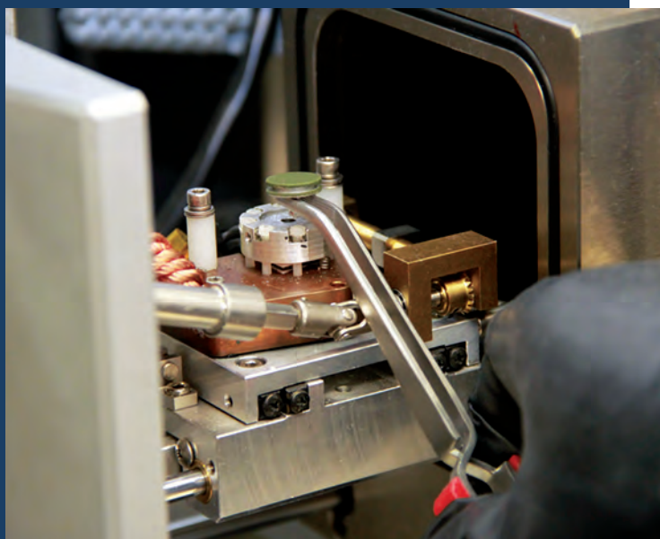
Close-up view of a painted sample (green colored stub held by tweezers) of a Chemical Agent Resistant Coating (CARC) being scanned using electron microscopy (SEM) and energy dispersive spectroscopy (EDS).
