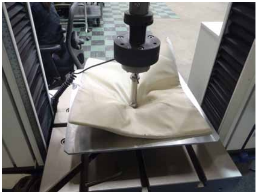
A Soft Armor Flexibility Test Apparatus measures armor sample stiffness by plunging it through an 8-inch diameter hole with a 2-inch depth. The new test is operationally relevant and is based on Soldier input regarding comfort and range of motion.
