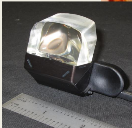
Free form molded prism with corrector
