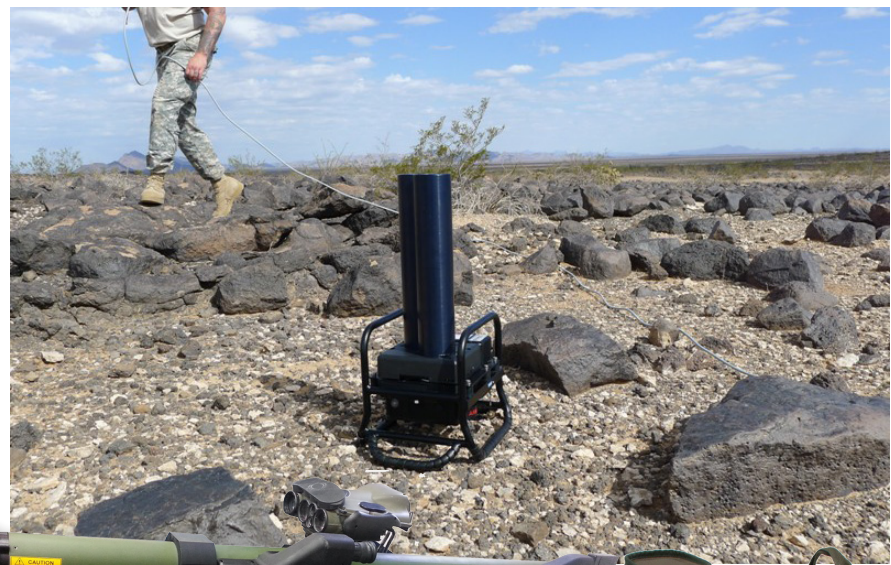
A Soldier prepares a simulator, which launches a self-consuming pyrotechnic pellet up to about 550 feet. (U.S. Army photos)
