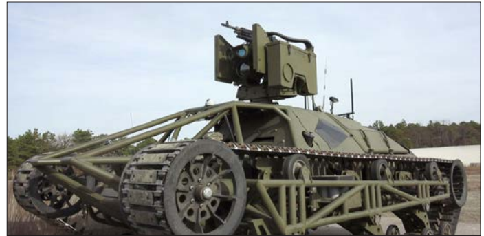
The Ripsaw Unmanned Ground Vehicle prepares to engage targets with an M240B mounted on a wirelessly controlled CROWS while conducting Scout Gunnery Table VI at Fort Dix, New Jersey, in November 2013. (U.S. Army photo)
