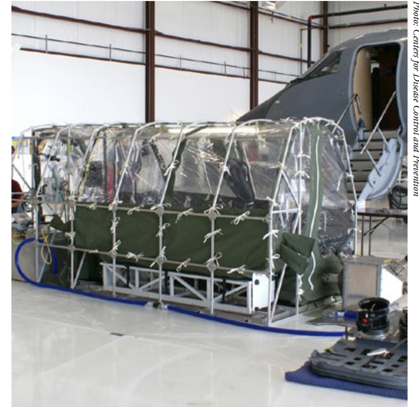
The Aeromedical Biological Containment System, which has been used to transport Ebola patients to the U.S. from West Africa, sits next to the Gulfstream III aircraft that carries it.
