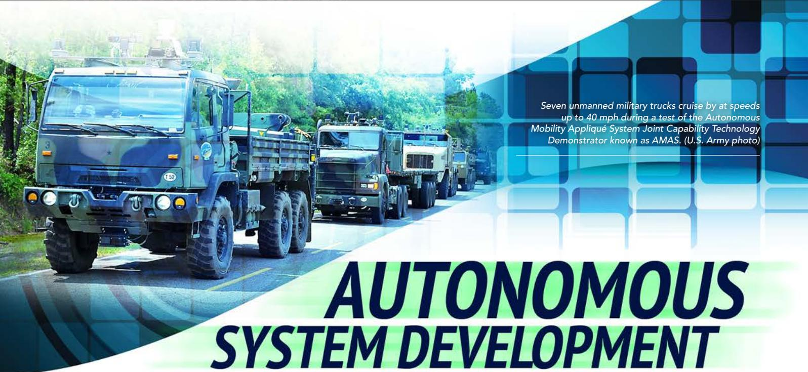
Seven unmanned military trucks cruise by at speeds up to 40 mph during a test of the Autonomous Mobility Appliqué System Joint Capability Technology Demonstrator known as AMAS. (U.S. Army photo)
