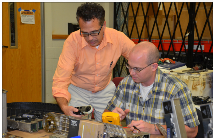
TARDEC Chief Engineer and Senior Technology Expert for Robotics Dr. Greg Hudas (standing) and TARDEC research scientist Jeremy Gray test circuit boards from a Packbot robot being completely refurbished at the center's Small Robots Laboratory. (U.S. Army photo by Amanda Dunford)
