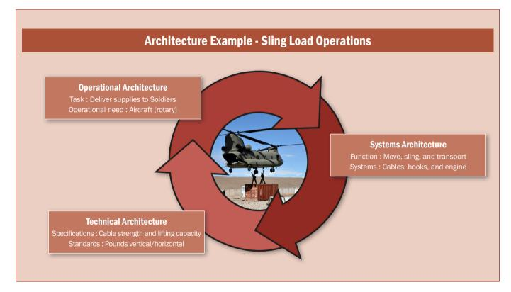
Figure 1. This provides examples of the items that might be used to complete each category for sling load operations architecture. Operational architecture is determined by the tasks or activities that must be performed. Systems architecture specifies the system functions and the systems that will be used to perform the operational activities. Technical architecture guides the systems selection for the operation.
