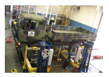
The SPIdER accurately characterizes vehicle suspension systems without modifying or disassembling most vehicles, and can apply both static and dynamic inputs to accurately measure multiaxle vehicle systems.
