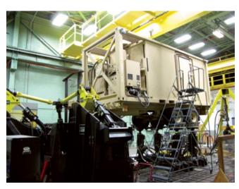
The PMBS is used to conduct durability and performance tests on lunette trailers. It provides motion and force inputs to the test trailer's tires and lunette to reproduce dynamic conditions experienced at proving grounds. The PMBS fatigues the trailer the way a field test would, but under controlled laboratory conditions.
