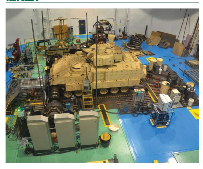
GVPM's Propulsion Test Cell 9 is a climatic chamber with wind capability equipped to evaluate continuous vehicle performance in extreme climates under full-load conditions.
