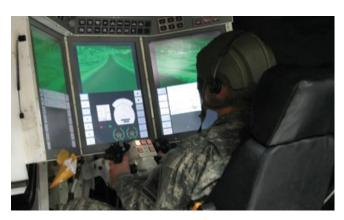
The CS/TMBS is a high-capacity six-degrees-of-freedom test device. The simulation framework enables engineers to quickly obtain key data and information on vehicle/Soldier performance with high quality. The simulator employs a virtual environment with computer-generated imagery and displays, a digital audio system, crew station controls, real-time computational dynamics and a network for synthetic battle-field operations.
