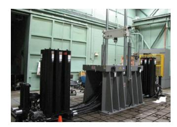
The STEM uses both durability and performance modes to determine the ability of shock absorbers or struts to withstand dynamic stress produced by transient waveforms. A key STEM characteristic, which exemplifies its one-of-a-kind nature, is its ability to achieve a minimum velocity of 5 meters per second at 20,000 lbs.
