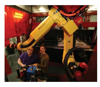
The RWL consists of a reconfigurable robotic arc welding cell and flexible tooling. This CSI lab also has hardware and software for writing welding programs.
