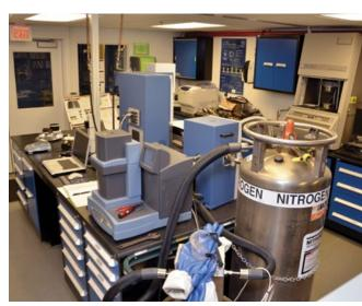
The Elastomer Lab performs research, development and testing to characterize elastomer components specific to track and suspension systems on legacy vehicles. Key objectives are characterization, failure mode analysis through benchmarking and screening current and improved materials. The team tests production materials for compliance and defines performance requirements for improved specifications. Results can be shared across other programs with elastomer, plastic and composite applications.
