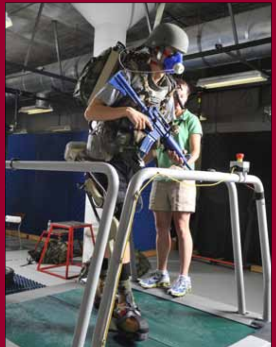
NSRDEC biomechanics research engineer Karen Gregorczyk (right) assesses the effects of the Ruggedized Human Universal Load Carriage, a lower-body exoskeleton, on the load carriage performance of a Soldier.
