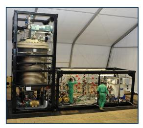
The Field Deployable Hydrolysis System was designed, developed and fabricated by a government team to provide a transportable, high throughput neutralization system designed to convert chemical warfare materiel into compounds not usable as weapons.
