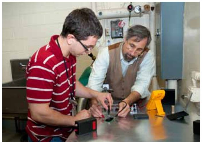
John Russo, who uses 3D printing to fabricate the Long-Lived Power battery casings, works with Dr. Marc Litz, both of the Power and Energy Division at ARL, to measure output voltage on space-grade photovoltaic cells before bonding tritium capsule to a photovoltaic wafer. (U.S. Army photo by Doug LaFon)
