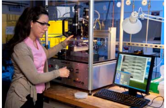
Dr. Sarah S. Bedair, an ARL electronics engineer, adjusts the settings on ink-jet printer used to deposit nanomaterials onto the surfaces of micro-devices. These devices would be used in high-power-density power supplies. The lab is pursuing energy solutions in areas like energy storage, alternative energy sources, high-density power converters and micro grids. (U.S. Army photo by Doug LaFon)
