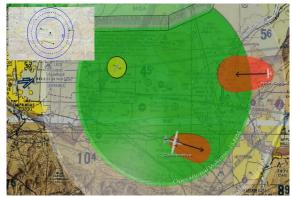
UAS maneuvers in air to ensure safe separation (no landing or return to restricted airspace required)
