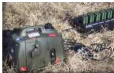
Honda 1kW generator modified to run on JP-8
