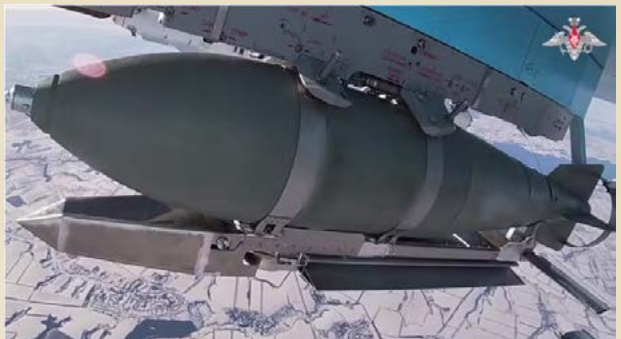
Screenshot of a video of a "high-explosive bomb" (HEB) equipped with the "UMPK" kit that makes it a guided glide bomb, released by the Russian Ministry of Defense, on its Telegram channel.
