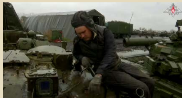
Whenever possible, repair points use modular repair by replacing faulty units with serviceable ones on hand or from captured Ukrainian equipment. (Russian Ministry of Defense)
