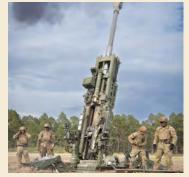
**M777** lightweight howitzers may not look particularly lightweight, but because they are made from titanium, they are 7,000 pounds lighter than the M198, which they replaced. They weigh around 9,500 pounds and have a maximum range of about 24 miles when firing their 105-pound 155mm shells. Currently being used in Ukraine, the Army has used the M777 since 2005.
