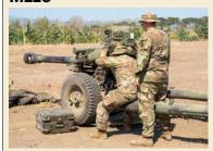
The **M119** is a smaller howitzer used by Infantry Brigades, particularly for air assault missions and was first used in Operation Desert Shield and Desert Storm in 1991 and is also seeing active use in Ukraine. It weighs around 4,700 pounds and has a range of about 12 miles when firing its 40-pound 105mm shells.
