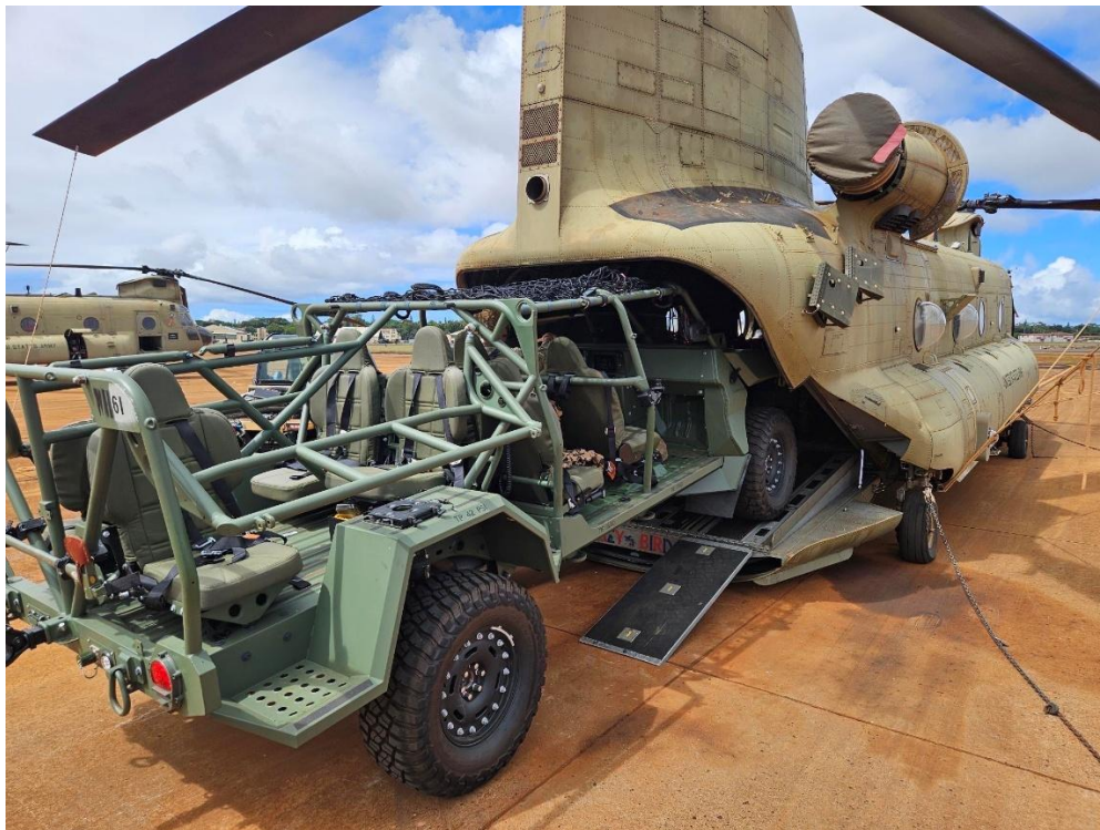
Figure 1: An Infantry Squad Vehicle is loaded onto an Army Chinook helicopter Photo Courtesy of the 225 th LSB, 25 th Infantry Division
