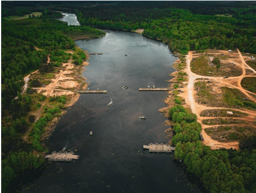
Figure 5: Overhead view of the Crossing Sites at the Drawsko Pomorski Combat Training Center. The 44rd MRBC has two rafts and the 23rd AMPH has two M3 Rigs in preparation for rafting or ferrying operations. Photo taken by MAJ Rafal Kazmierczyk, 11 May 2024 5 .
