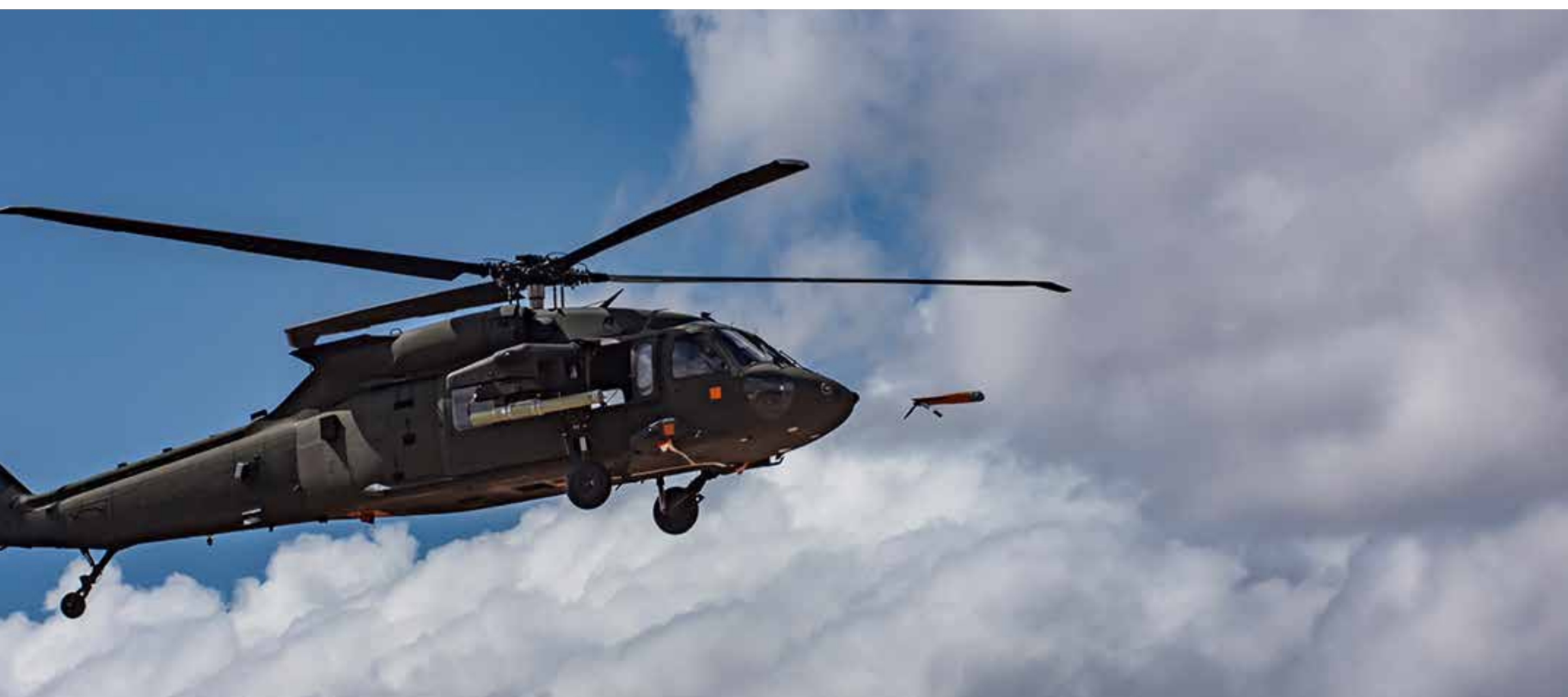
Air Launched Effects Demonstration: Area-I Agile-Launched, Tactically Integrated, Unmanned System (ALTIUS) horizontal launch from a UH-60.
