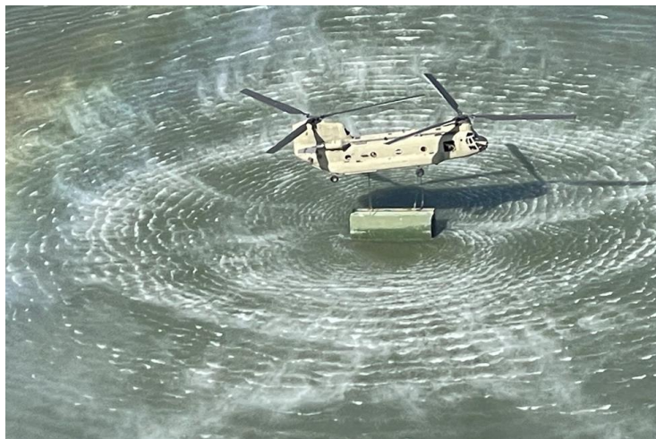
B 2/238 GSAB sling loading IRB bays onto the Arkansas River in support of the 1140 th EN BN Gap Crossing.
