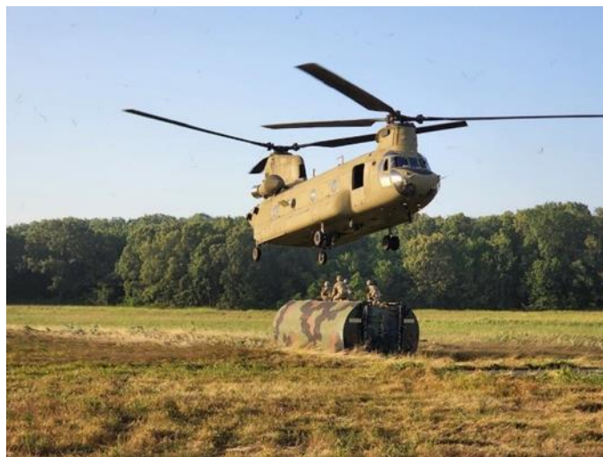
B 2/238 GSAB sling loading IRB bays onto the Arkansas River in support of the 1140 th EN BN Gap Crossing. (FORT CHAFFEE)
