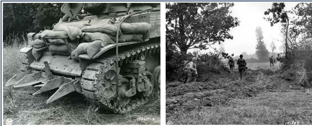
Figure 1. Allied “Rhino Tank” with steel tusks/bocage cutting device attached and a cleared path through a bocage hedgerow in France during World War II. 3
