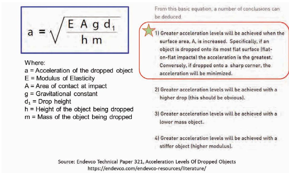
FIGURE 2 Container drop orientation upon maximum G's experienced during drop tests
