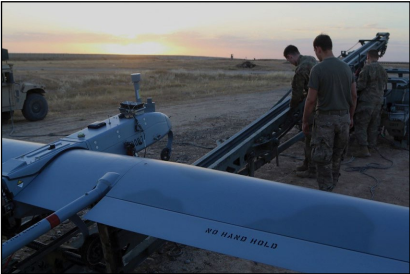
Figure C-5. Soldiers assigned to the 4th Squadron, 6th Cavalry Regiment, 16th Combat Aviation Brigade, prepare to launch a RQ-7B Shadow Tactical Unmanned Aircraft System, 22 May 2017. (Photo by SSG Heidi McClintock, U.S. Army)
