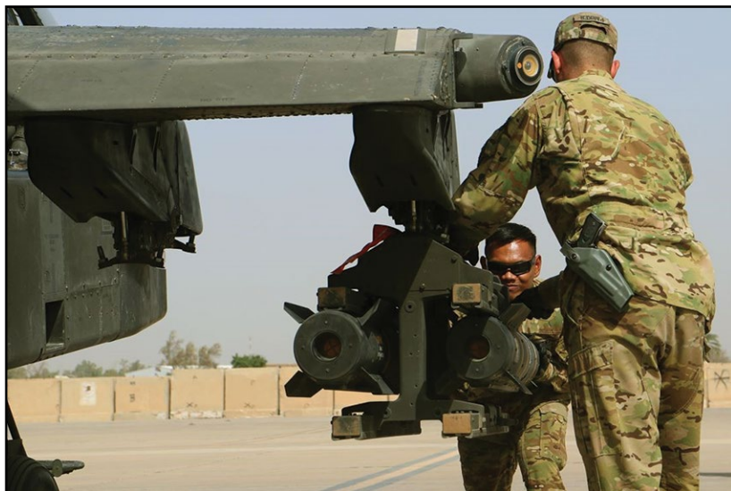
Figure 1-8. Soldiers slide a Hellfire missile into place on an AH-64 Apache attack helicopter in Iraq. (Photo by SFC R.W. Lemmons IV, U.S. Army)
