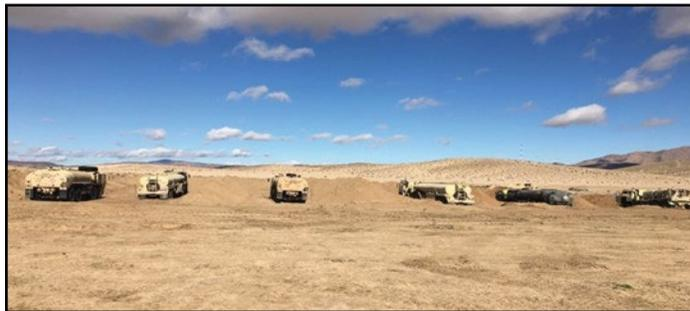
**Figure 10-3. Example tanker spacing. Tanker spacing directly contributes to commodity protection.**
