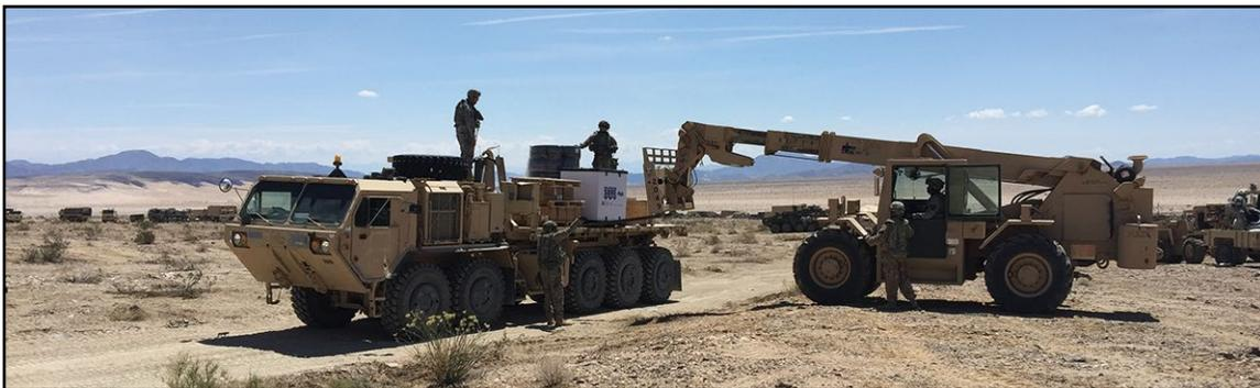
**Figure 19-2. An example of inefficient flatrack unloading using a forklift from a Palletized Load System Flat-rack. It's better to drop the flatrack and pick up an empty one.**
