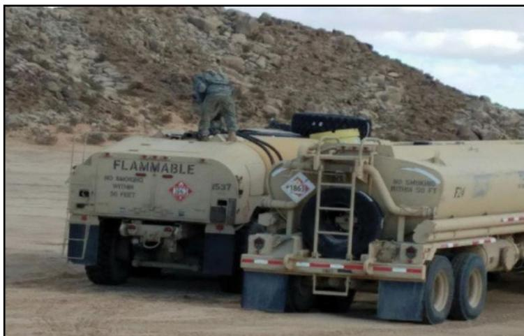
**Figure 10-4. Fueler top loading. BII shortages can cause a 15x time delay in fueling operations.**
