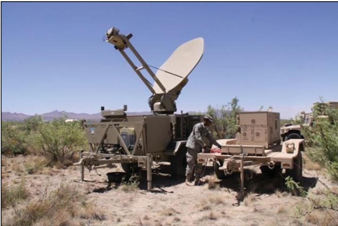
**Figure 16-3. Satellite Transmission Terminal (STT).**
