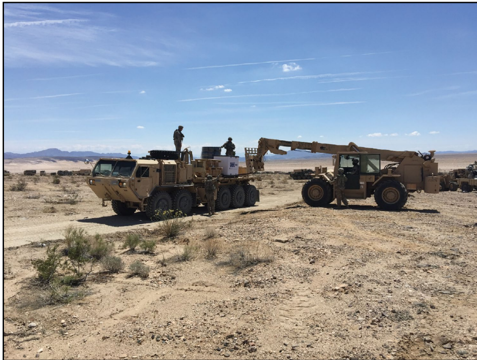
Figure 10-13. Using a forklift to unload items from a palletized load system flatrack is not efficient. A better way is to drop the flatrack and pick up an empty one.
