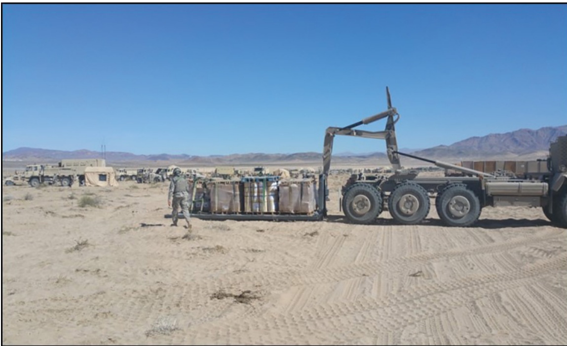
Figure 12-2. Flat rack exchange conducted at a CTCP.
