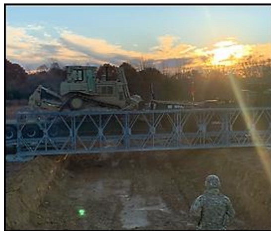
LET with D7 crosses LOC-B ACROW Bridge during a 19th EN BN FTX (20th EN BDE)
