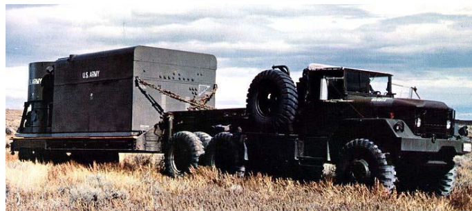
The U.S. Army's Mobile Low-Power First Generation (ML-1) MNPP from the early 1960s
