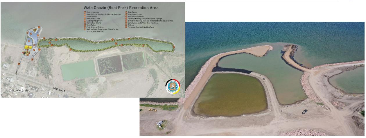
The project is designed to abate erosion that poses an imminent threat to the Lower Brule sewage lagoons and the town's infrastructure, and to address habitat degradation that has occurred along the shoreline of Lake Sharpe.
