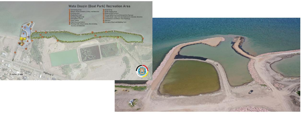
The project is designed to abate erosion that poses an imminent threat to the Lower Brule sewage lagoons and the town's infrastructure, and to address habitat degradation that has occurred along the shoreline of Lake Sharpe.
