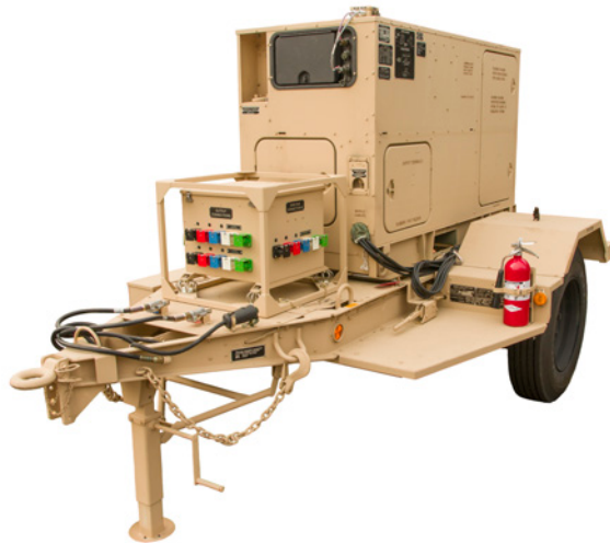
Military-standard AMMPS 60kW generator with microgrid switchbox mounted on a trailer. Up to six 60kW generators can be networked into a microgrid. (U.S. Army photo courtesy of PM E2S2.)
